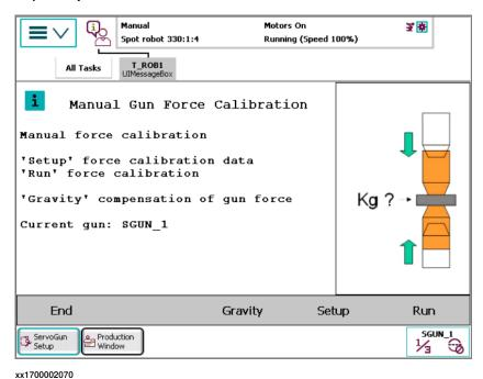
3 By default, the force calibration is performed by doing two force measurements (typically at half max force and at max force). To change number of measurements, tap 1 and then enter the number of measurements. To change the max force that the servo gun shall reach, tap 2 and then enter the new value.
