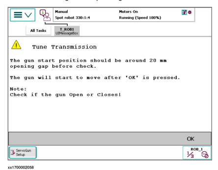
3 Observe the direction of the movement. If the gun opened, tap **Open**. If the gun closed, tap **Close**.
