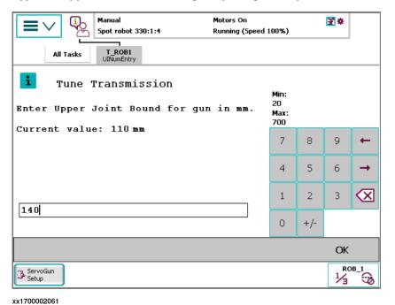
6 Measure the gun opening. If it is not exactly 50 mm, tap **No** and type the measured value.
