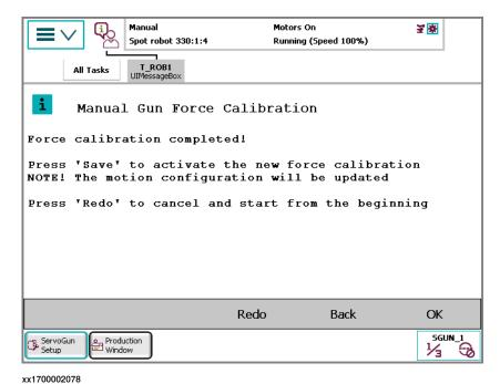
13 Repeat step 4 to 12 until the max force has been reached (typically 2-3 times). Then tap **End**.
